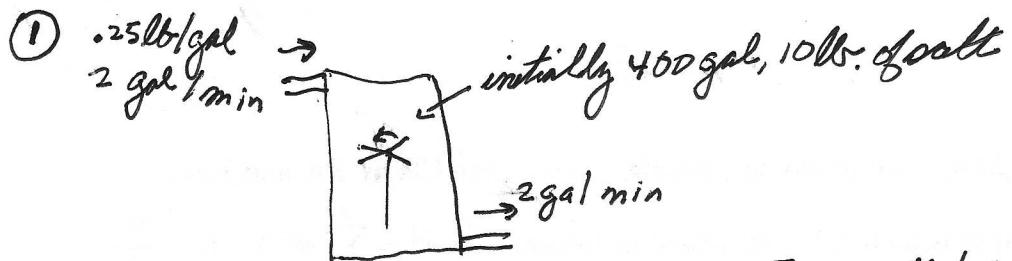
$$[\text{Rate in}] = [(0.25) \text{ lb/gal}] [2 \text{ gal/min}] = 0.5 \text{ lb/min}$$
