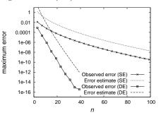
Figure 4: Error of Sinc indefinite integration for (4.4) and its estimate.
